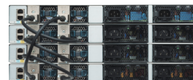
Catalyst 9200 Modular Uplink Models Stacked using optional StackWise-160 Kits, 2 PSU (optional 2nd PSU installed)
