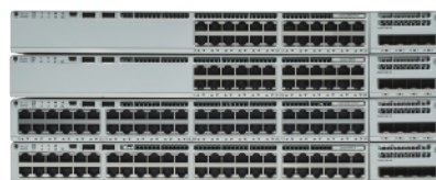
Catalyst 9200 Modular Uplink Models Stacked using optional StackWise-160 Kits, 2 PSU (optional 2nd PSU installed)
